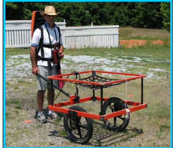
The photograph shows the Geonics EM61 metal detector that was used to conduct the metal detection survey across the City of Greenville property (Parcel 186) on August 22, 2012.
