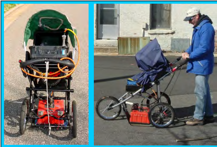
The photographs show the SIR-2000 GPR system equipped with a 400 MHz antenna that were used to conduct the ground penetrating radar investigation across selected EM61 differential anomalies at the Parcel 186 site on August 29, 2012.
