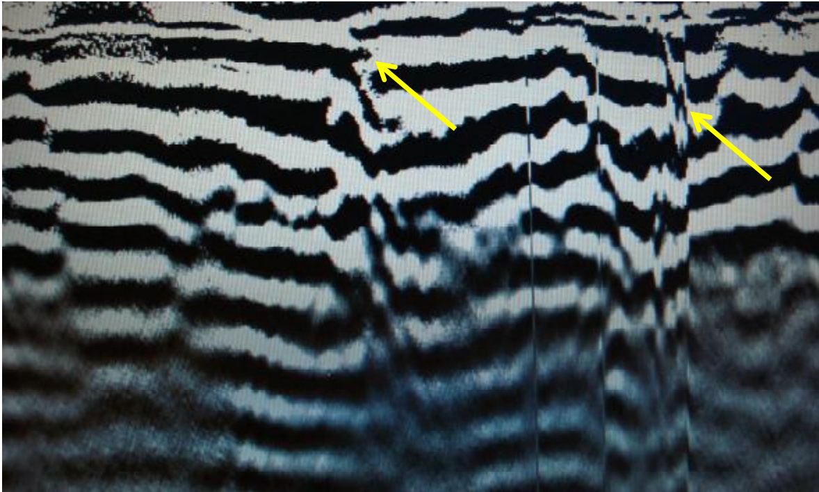
Two sets of parallel anomalies. First set of water lines and second of drain lines for storm water
