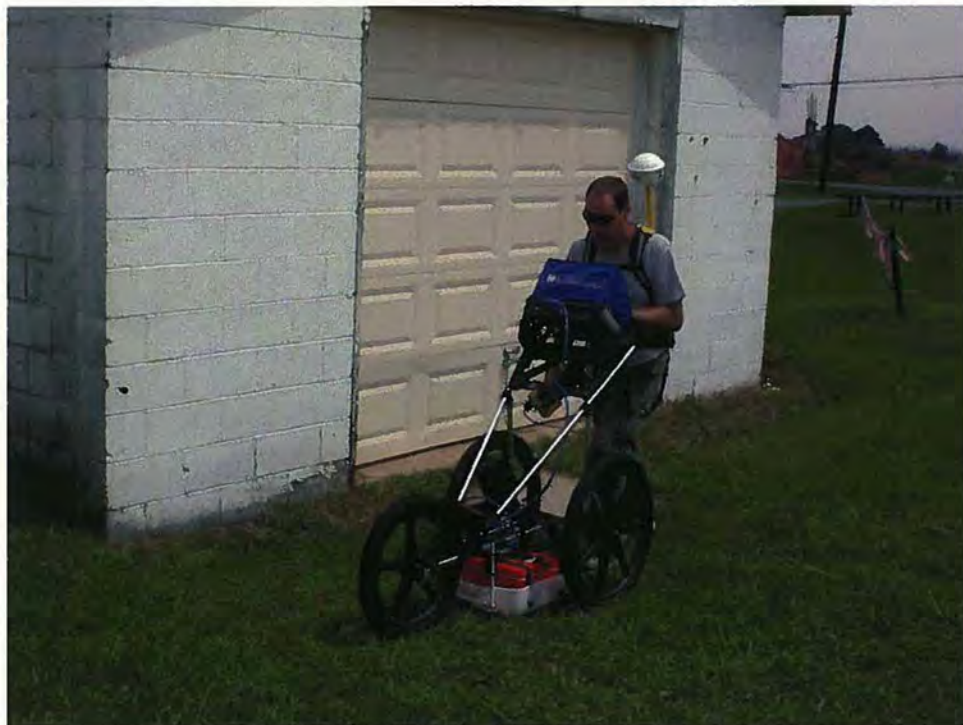
GSSI SIR-3000 Ground-Penetrating Radar with 400 MHz Antenna
