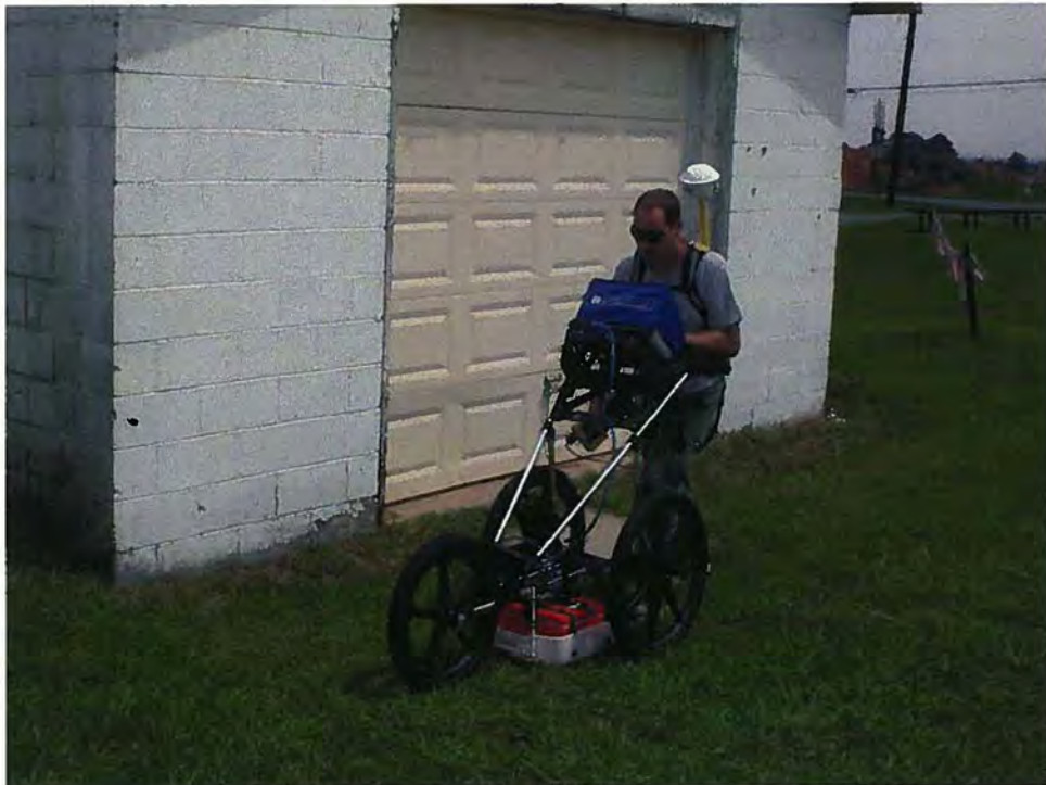
GSSI SIR-3000 Ground-Penetrating Radar with 400 MHz Antenna
