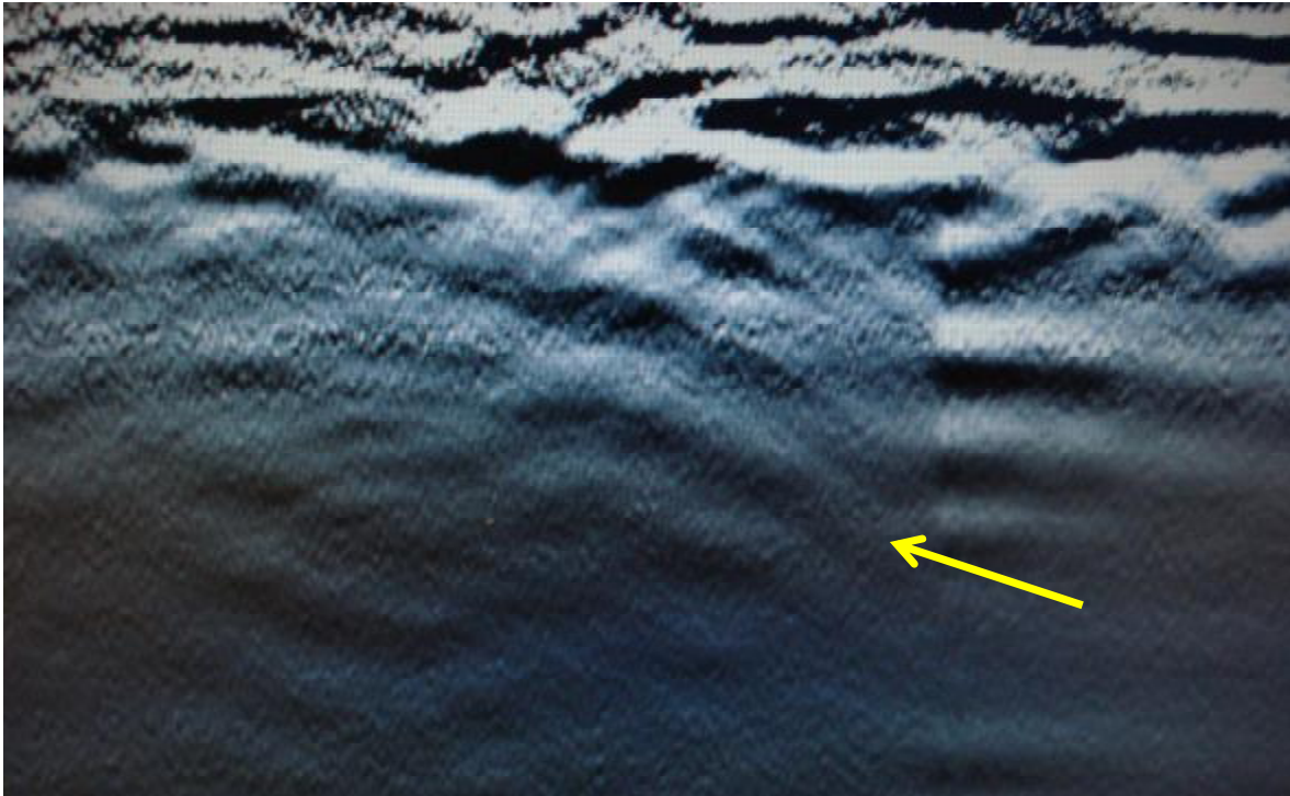
GPR READINGS SHOWING SOIL DIFERENTIATIONS AT WALLS OF PROBABLE UST AND HYPERBOLAE WITH METAL CONTENT INCLUDING NEAR SPIKE FROM VENT PIPES
