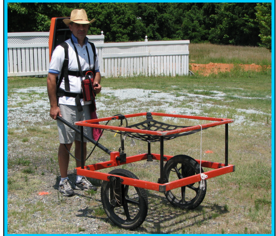
The photograph shows the Geonics EM61 metal detector that was used to conduct the metal detection survey across the Blount, et al property (Parcel 13) on August 15, 2012.
