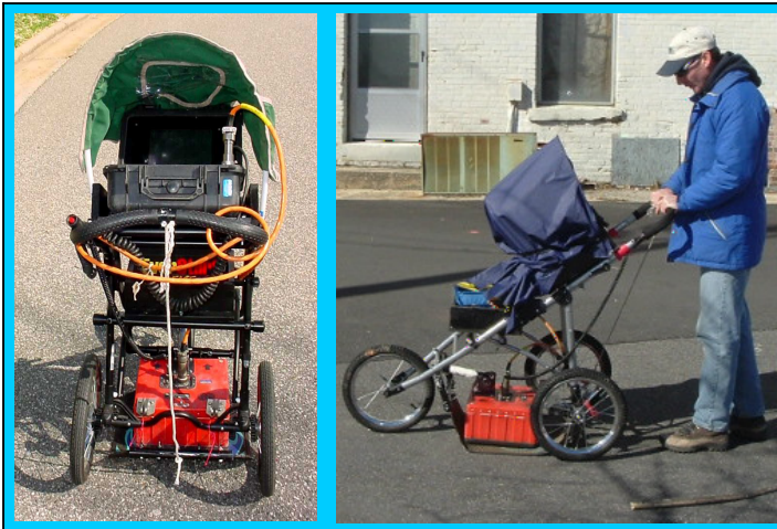
The photographs show the SIR-2000 GPR system equipped with a 400 MHz antenna that were used to conduct the ground penetrating radar investigation across selected EM61 differential anomalies at the Parcel 13 site on August 21, 2012.
