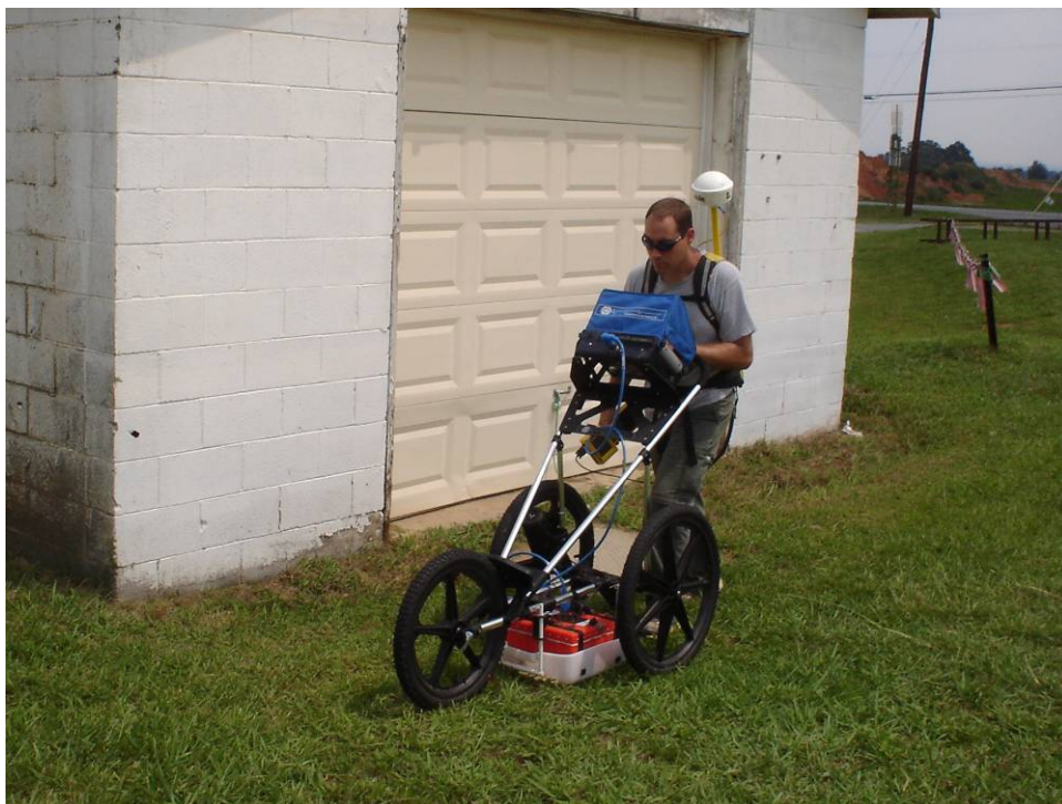
GSSI SIR-3000 Ground-Penetrating Radar with 400 MHz Antenna
