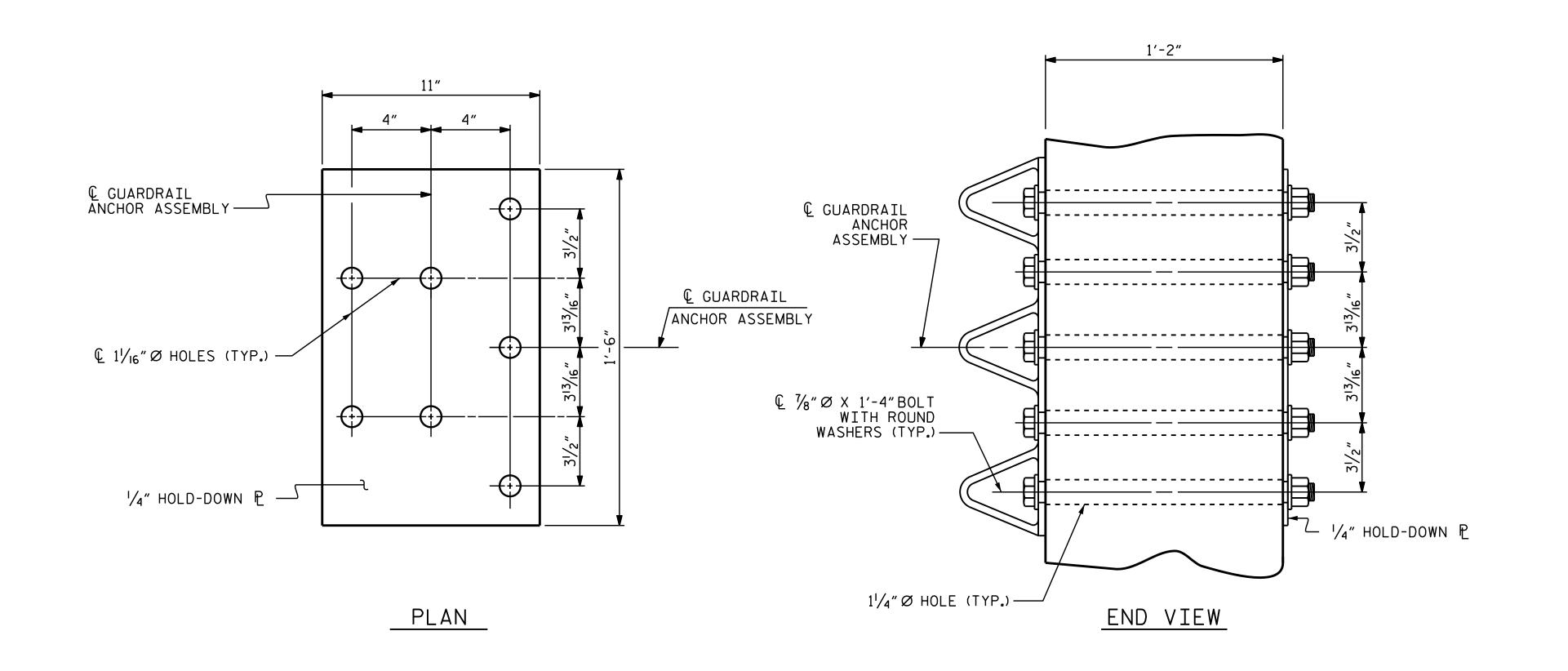
GUARDRAIL ANCHOR ASSEMBLY DETAILS
