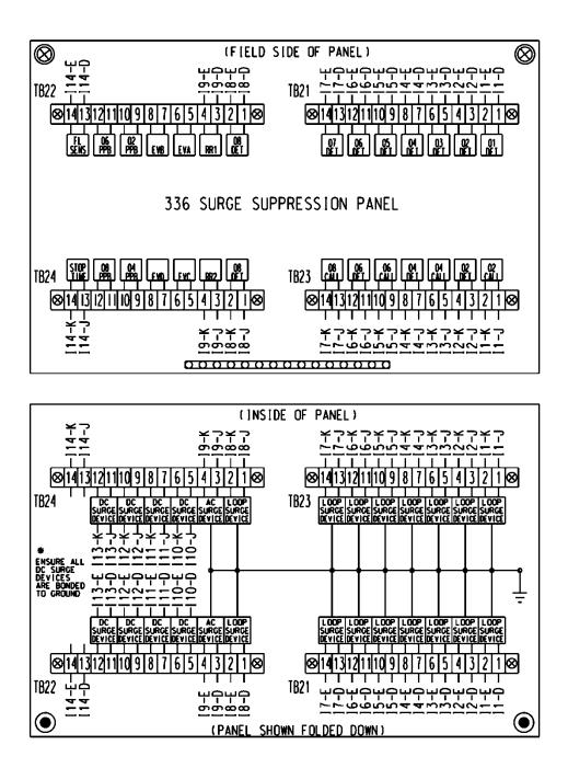
Provide permanent labels that indicate the slot and the pins connected to each terminal that may be viewed from the rear cabinet door. Label and orient terminals so that each pair of inputs is next to each other. Indicate on the labeling the input file (I or J), the slot number (1-14) and the terminal pins of the input slots (either D & E for upper or J & K for lower).
