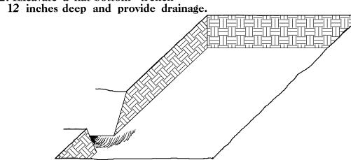
3. Backfill the trench with 2 inches well rotted sawdust. Place a 2 inch layer of well rotted sawdust at a sloping angle
