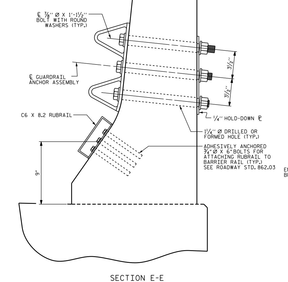
GUARDRAIL ANCHOR ASSEMBLY DETAILS
