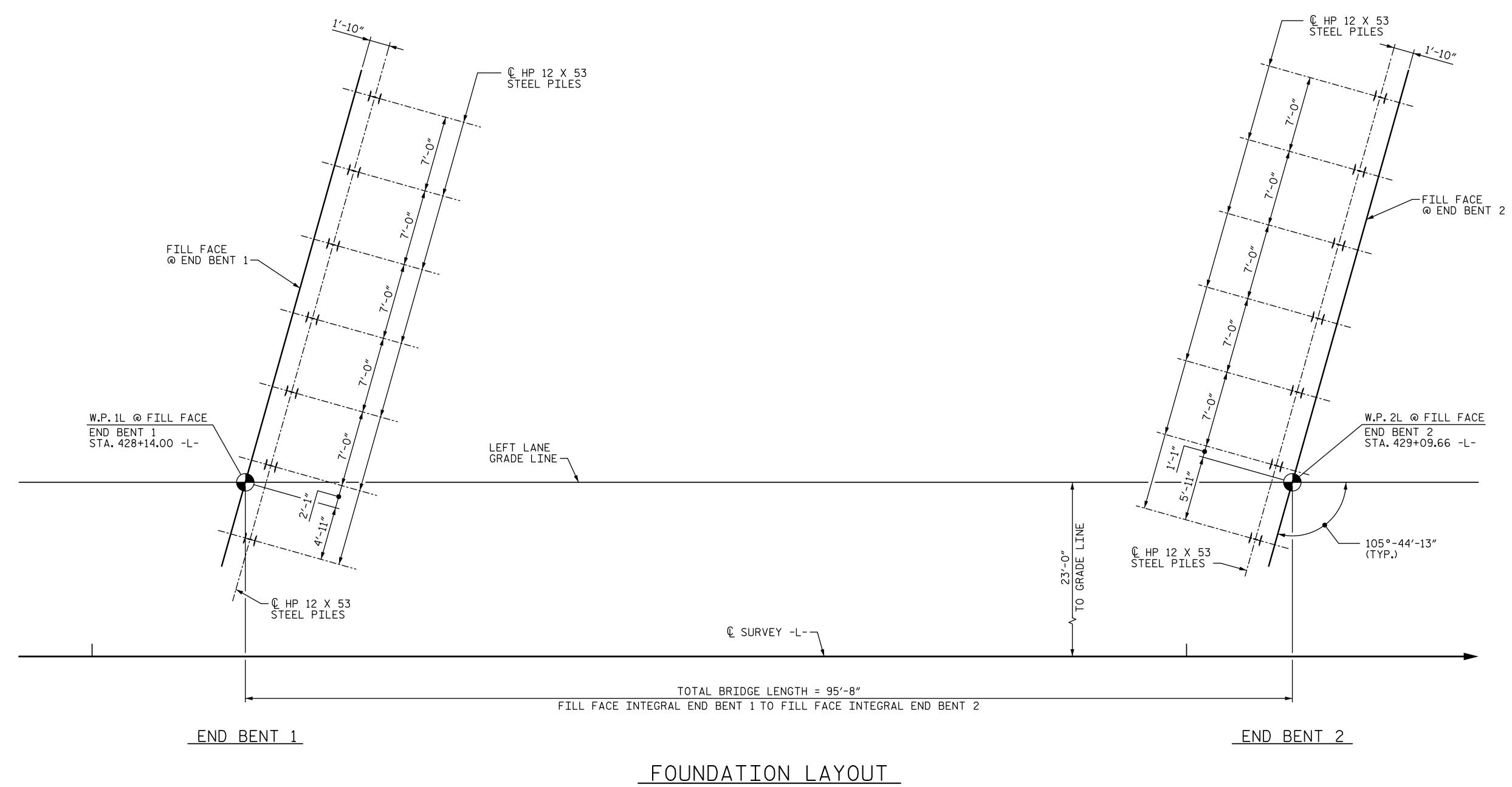
(DIMENSIONS LOCATING PILES ARE SHOWN TO THE PILE CENTERLINE.)
