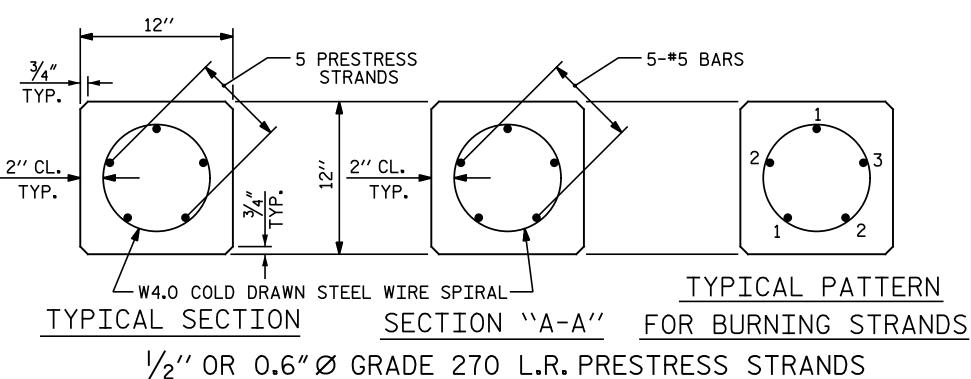
4 PRESTRESS 4- #5 BARS **STRANDS** TYP. 2" CL. TYP. TYPICAL PATTERN ∠ W4.0 COLD DRAWN STEEL WIRE SPIRAL TYPICAL SECTION SECTION "A-A" FOR BURNING STRANDS 1/2" OR 0.6" Ø GRADE 270 L.R. PRESTRESS STRANDS
