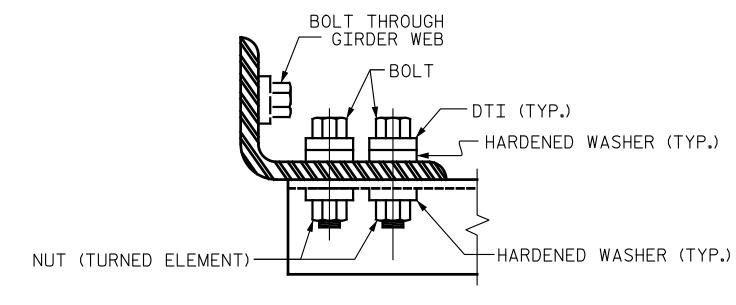
BOLT WITH DTI ASSEMBLY DETAIL
