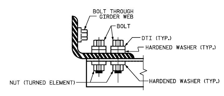
BOLT WITH DTI ASSEMBLY DETAIL
