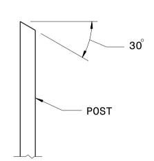
DETAIL SHOWING METHOD OF CUTTING POST TOPS
