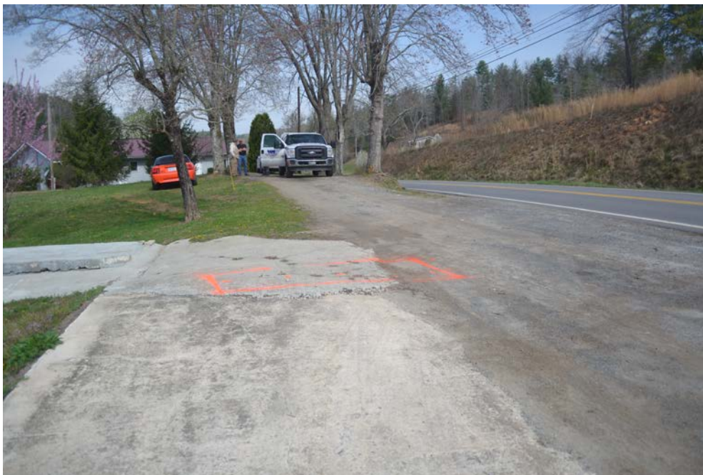
Photograph 2: Potential UST identified at NCDOT Parcel 23 by GPR and demarcated in orange paint on April 4, 2014. View is to the northwest parallel to NC 294. Gravel drive extends to the Tammy Wood Wright residence, which can be seen in background.
