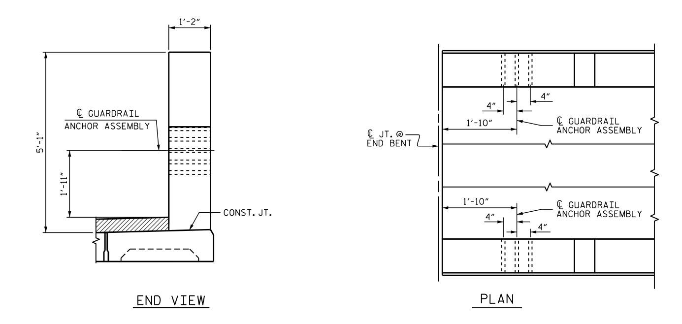
LOCATION OF GUARDRAIL ANCHOR AT END POST
