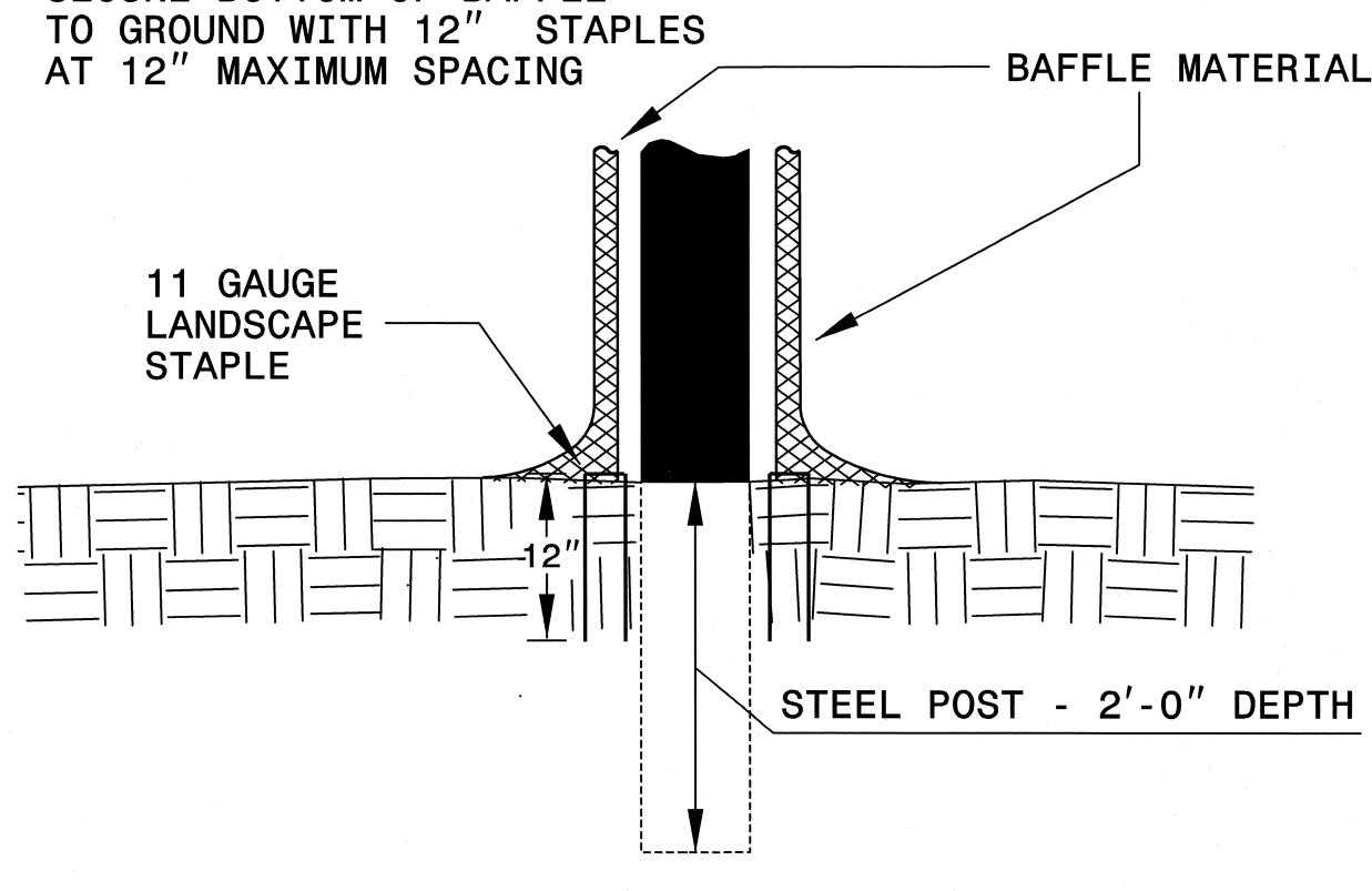
BAFFLE MATERIAL SHALL BE SECURED TO THE BOTTOM AND SIDES OF BASIN USING 12" LANDSCAPE STAPLES
