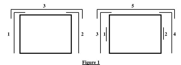
Cover the external joint sealer with a 3 foot strip of filter fabric conforming to Type 4 requirements in Section 1056 of the Standard Specifications.
