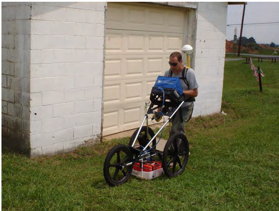
GSSI SIR-3000 Ground-Penetrating Radar with 400 MHz Antenna
