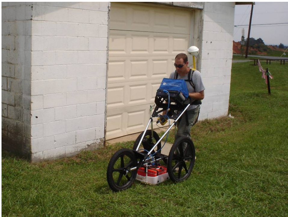
GSSI SIR-3000 Ground-Penetrating Radar with 400 MHz Antenna
