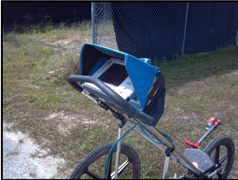
5 GPR unit adjacent to former AST enclosure.
