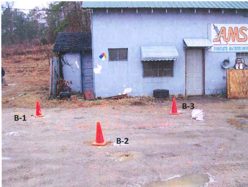
Photo #1: Location of probable USTs and borings B-1 through B-3 at southeast building corner.
