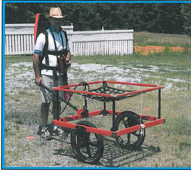
The photograph shows the Geonics EM61 metal detector that was used to conduct the metal detection survey across the proposed Right-of-Way area at Parcel 197 on November 11, 2011. Due to an absence of unexplained EM61 differential anomalies, ground penetrating radar scans were not performed at this site.
