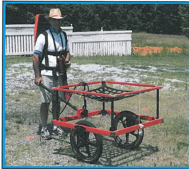
The photograph shows the Geonics EM61 metal detector that was used to conduct the metal detection survey across the proposed Right-of-Way area at Parcel 193 on November 10, 2011. Due to an absence of unexplained EM61 differential anomalies, ground penetrating radar scans were not performed at this site.
