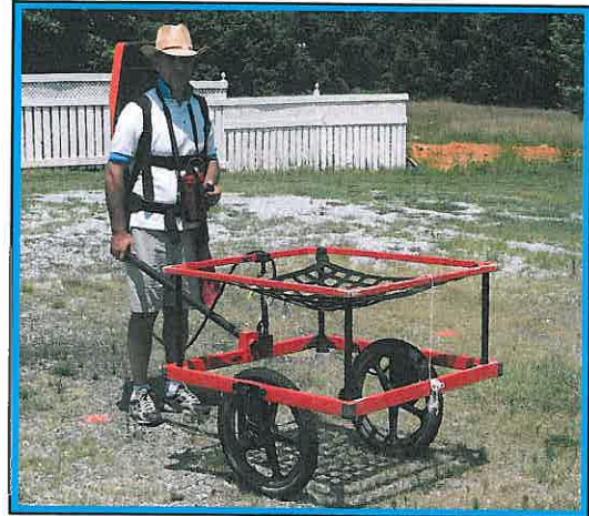
The photograph shows the Geonics EM61 metal detector that was used to conduct the metal detection survey across the proposed Right-of-Way area at Parcel 181 on November 10, 2011.
