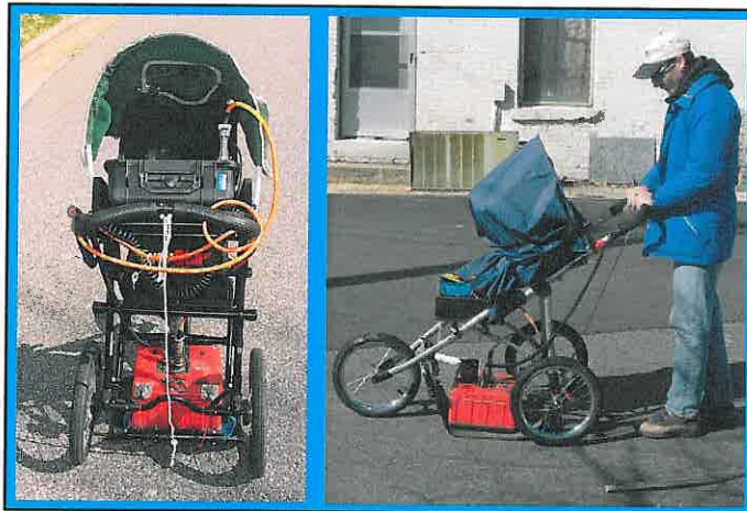
The photographs show the SIR-2000 GPR system equipped with a 400 MHz antenna that were used to conduct the ground penetrating radar investigation across selected EM61 differential anomalies at Parcel 181 on November 17, 2011.
