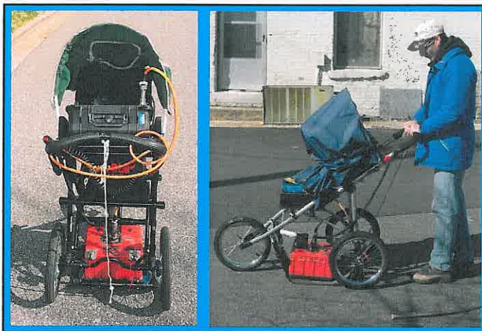
The photographs show the SIR-2000 GPR system equipped with a 400 MHz antenna that were used to conduct the ground penetrating radar investigation across selected EM61 differential anomalies at Parcel 167 on November 17, 2011.
