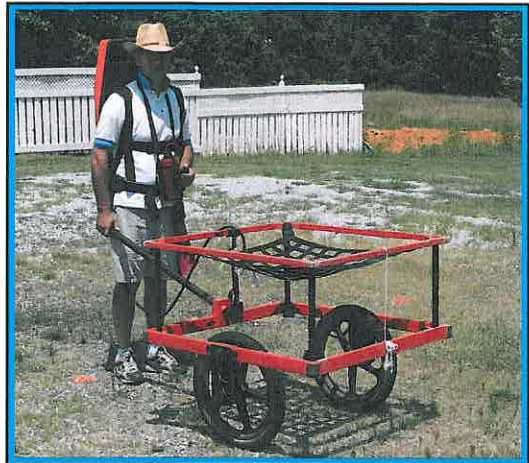
The photograph shows the Geonics EM61 metal detector that was used to conduct the metal detection survey across the proposed Right-of-Way area at Parcel 167 on November 10, 2011.
