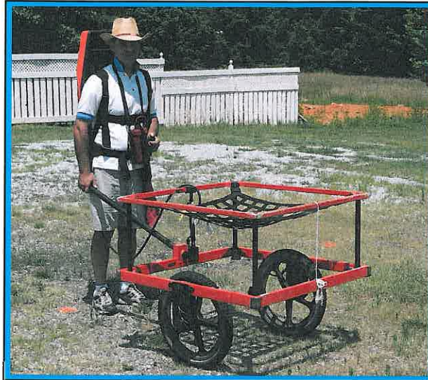
The photograph shows the Geonics EM61 metal detector that was used to conduct the metal detection survey across the proposed Right-of-Way area at Parcel 150 on November 10, 2011. Due to an absence of unexplained EM61 differential anomalies, ground penetrating radar scans were not performed at this site.
