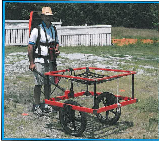
The photograph shows the Geonics EM61 metal detector that was used to conduct the metal detection survey across the proposed Right-of-Way area at Parcel 145 on November 10, 2011. Due to an absence of unexplained EM61 differential anomalies, ground penetrating radar scans were not performed at this site.
