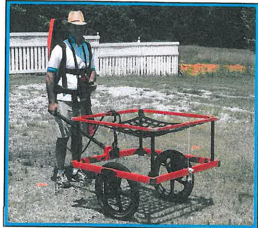
The photograph shows the Geonics EM61 metal detector that was used to conduct the metal detection survey across the proposed Right-of-Way area at Parcel 111 on November 9, 2011.
