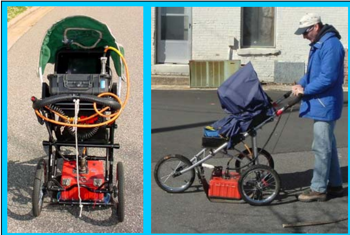
The photos show the SIR-2000 GPR system equipped with a 400 MHz antenna that were used to conduct the ground penetrating radar investigation at Parcel 48 on June 27, 2007.
