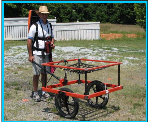
The photo shows the Geonics EM61 metal detector that was used to conduct the metal detection survey at Parcel 11 on June 21, 2007.
