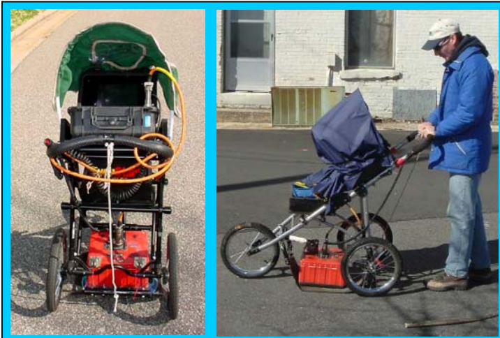
The photos show the SIR-2000 GPR system equipped with a 400 MHz antenna that were used to conduct the ground penetrating radar investigation at Parcel 11 on June 26, 2007.
