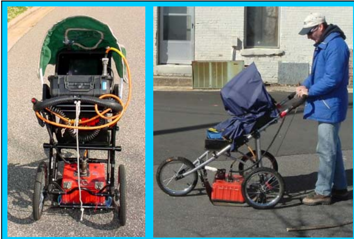
The photos show the SIR-2000 GPR system equipped with a 400 MHz antenna that were used to conduct the ground penetrating radar investigation at Parcel 9 on June 26, 2007.
