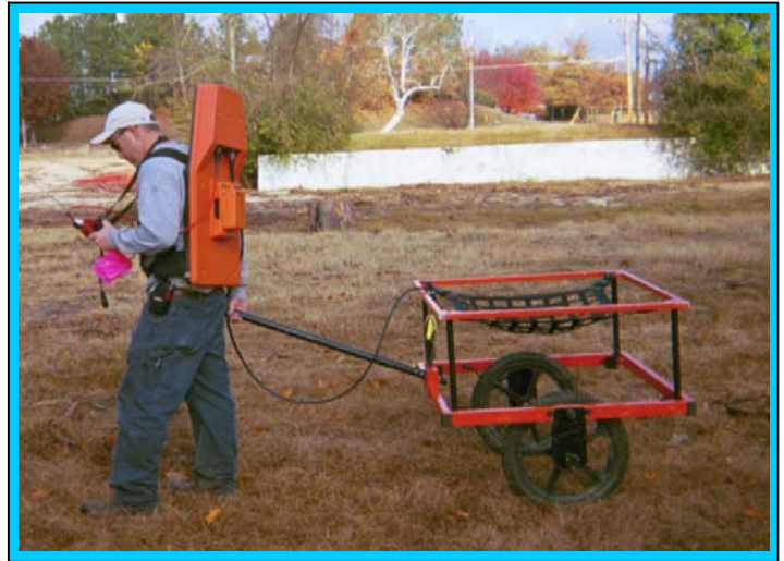
The photo shows the Geonics EM61 metal detector that was used to conduct the metal detection survey at Parcel 49 on June 21, 2007.
