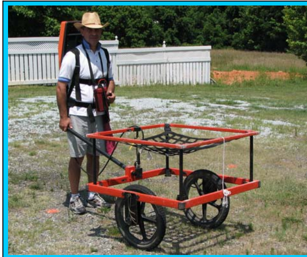
The photo shows the Geonics EM61 metal detector that was used to conduct the metal detection survey at Parcel 7 on June 22, 2007.
