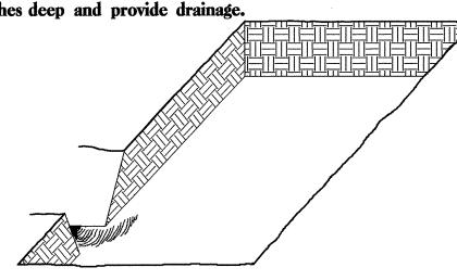
3. Backfill the trench with 2 inches well rotted sawdust. Place a 2 inch layer of well rotted sawdust at a sloping angle at one end of the trench.
