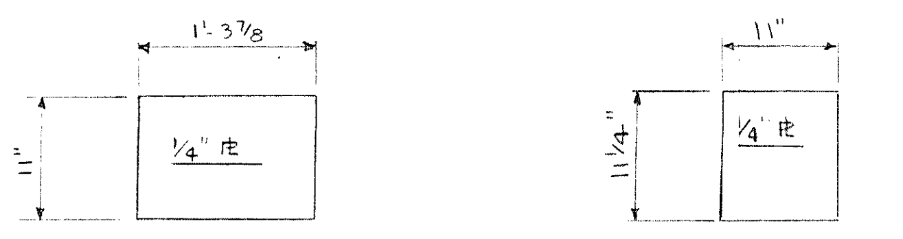
TOP & BOTTOM PLATES (4 REQUIRED) END PLATES (4 REQUIRED) CONDUIT SLEEVE DETAILS (2 SLEEVES REQUIRED)
