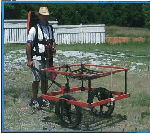
The photograph shows the Geonics EM61 metal detector that was used to conduct the metal detection survey across the geophysical survey area at the St. Horore Investments property (Parcel 139) on June 24, 2010.
