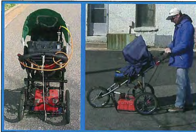
The photographs show the SIR-2000 GPR system equipped with a 400 MHz antenna that were used to conduct the ground penetrating radar investigation at Parcel 132 on July 1, 2010.
