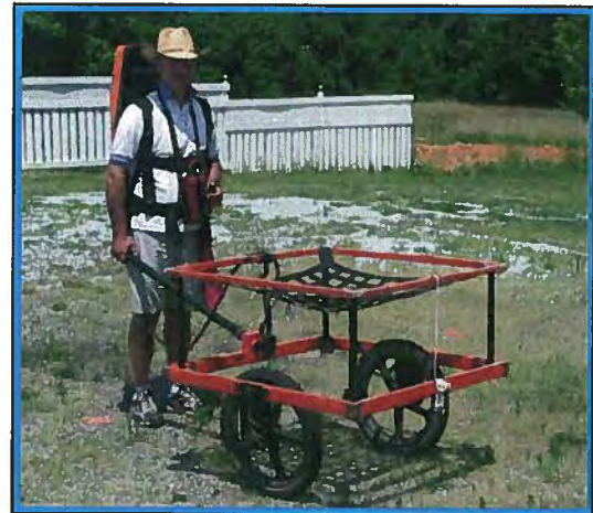
The photograph shows the Geonics EM61 metal detector that was used to conduct the metal detection survey across the southwestern portion of Parcel 132 on June 25, 2010.
