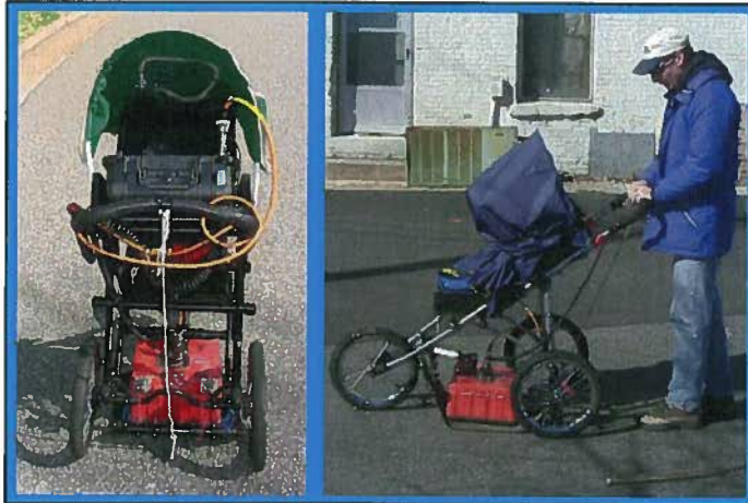
The photographs show the SIR-2000 GPR system equipped with a 400 MHz antenna that were used to conduct the ground penetrating radar investigation at Parcel 125 on July 1, 2010.
