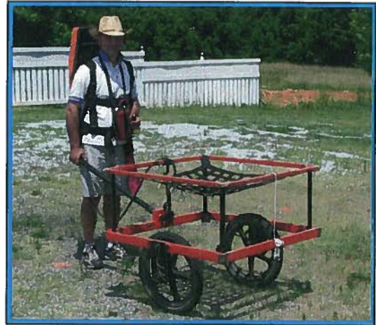
The photograph shows the Geonics EM61 metal detector that was used to conduct the metal detection survey across the area of interest at Parcel 125 on June 28, 2010.
