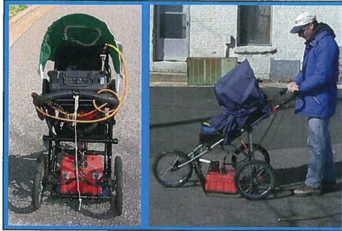
The photographs show the SIR-2000 GPR system equipped with a 400 MHz antenna that were used to conduct the ground penetrating radar investigation at Parcel 119 on June 29, 2010.
