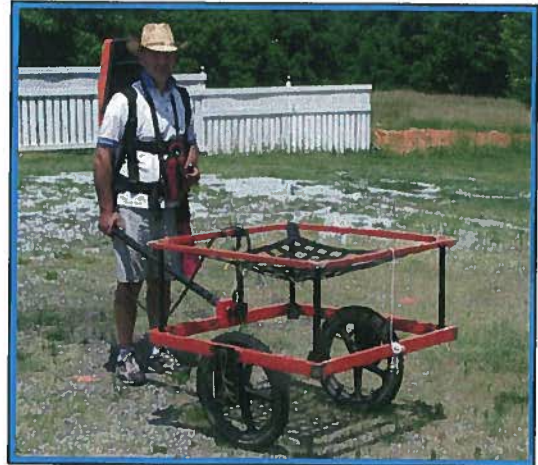
The photograph shows the Geonics EM61 metal detector that was used to conduct the metal detection survey across Parcel 107 on June 23, 2010.
