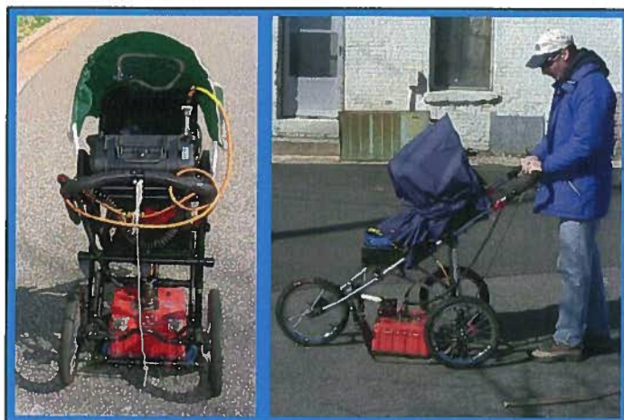
The photographs show the SIR-2000 GPR system equipped with a 400 MHz antenna that were used to conduct the ground penetrating radar investigation at Parcel 107 on July 1, 2010.
