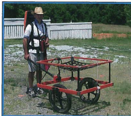
The photograph shows the Geonics EM61 metal detector that was used to conduct the metal detection survey across Parcel 107 on June 23, 2010.
