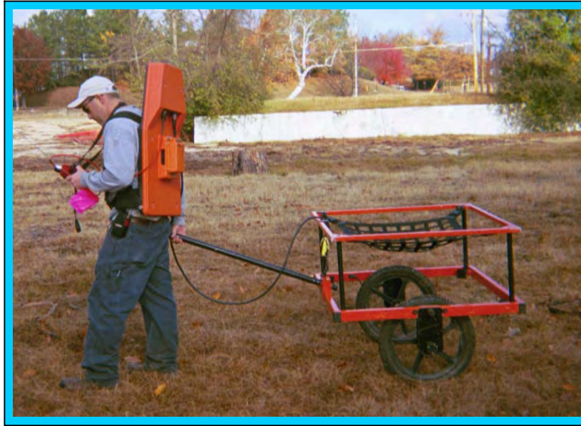
The photo shows the Geonics EM61 metal detector that was used to conduct the metal detection survey at the Old South Main Street and East "A" Avenue sites in Salisbury, North Carolina on June 26, 27, and July 7, 2006. The instrument has a maximum investigating depth of approximately 8 feet.
