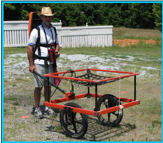
The photograph shows the Geonics EM61 metal detector that was used to conduct the metal detection survey across the proposed ROW area at the Waymon Parker property on July 21, 2010.
