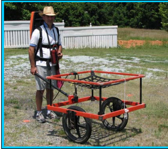
The photograph shows the Geonics EM61 metal detector that was used to conduct the metal detection survey across the proposed ROW area at the Helen Faircloth Properties Inc. site on July 22, 2010.
