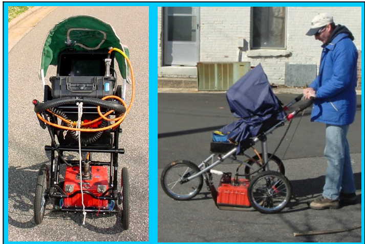
The photographs show the SIR-2000 GPR system equipped with a 400 MHz antenna that were used to conduct the ground penetrating radar investigation at the Roy Byrd property on August 2, 2010.
