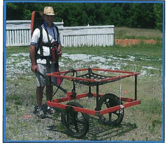
The photograph shows the Geonics EM61 metal detector that was used to conduct the metal detection survey at Parcel 22 on October 22, 2010.
