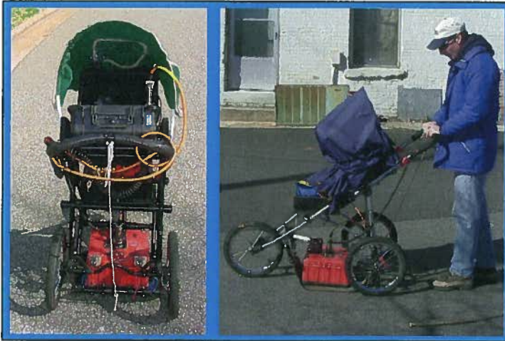
The photographs show the SIR-2000 GPR system equipped with a 400 MHz antenna that were used to conduct the ground penetrating radar investigation at Parcel 22 on October 29, 2010.
