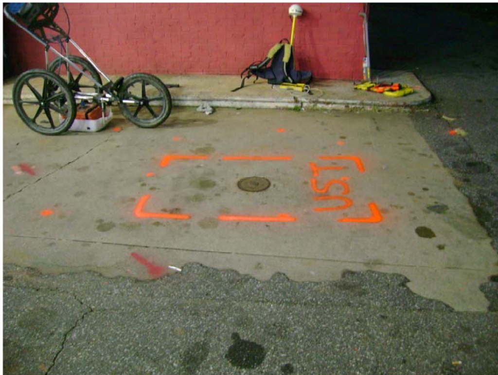
Parcel 34 – KHT & H, LLC Property, looking east. Photo shows approximate marked location of a probable UST near the southwestern corner of the building.
